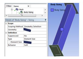
To the blue parts assign this Mesh Sizing.
