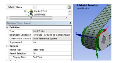
After the solving is done, click Solution, then Worksheet button to access these extra results for Angle, Angular Velocity and Angular Acceleration.
