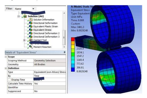
Create a Directional Deformation for the lateral faces of the workpiece.
