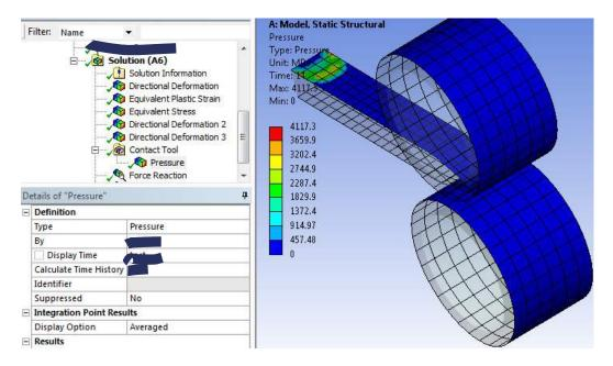
From Probe, Force Reaction and Moment Reaction, insert these items.
