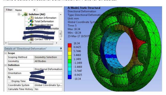
Insert an Equivalent Stress only for the cage.
