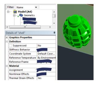
To the outer shell bodies, green here, apply CTTTL and Thickness = 1 mm.
