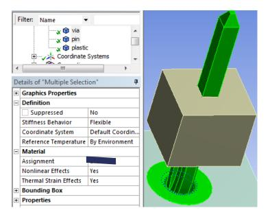
Assign PBT GF30 material on the via and pin, green here.
